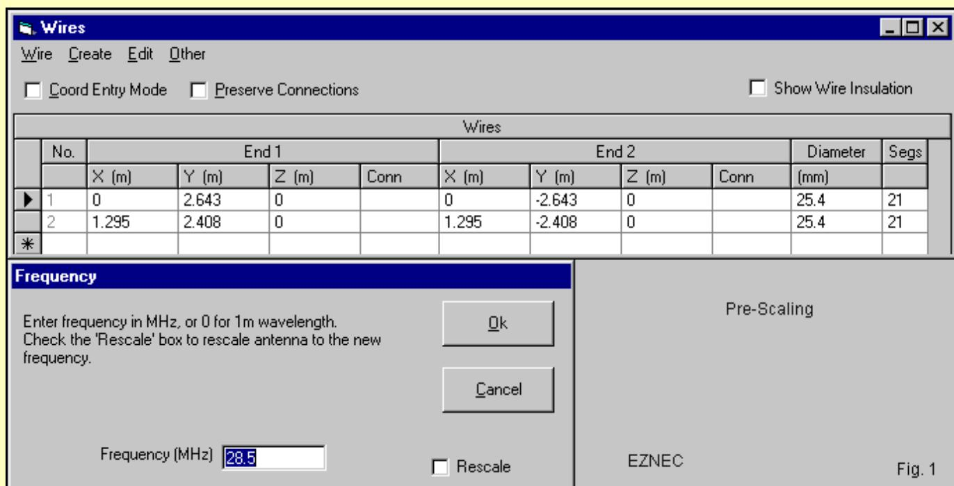
EZNEC implements scaling through the frequency selection screen. Note the box marked "Rescale." Let's revise the frequency to 14.25 MHz and also click on the rescale box. The result will be the set of wire entries shown in **Fig. 2**. The user made none of the changes in the wire tables. Rather, the program made the necessary changes after the user entered the new frequency and checked the rescale box.
